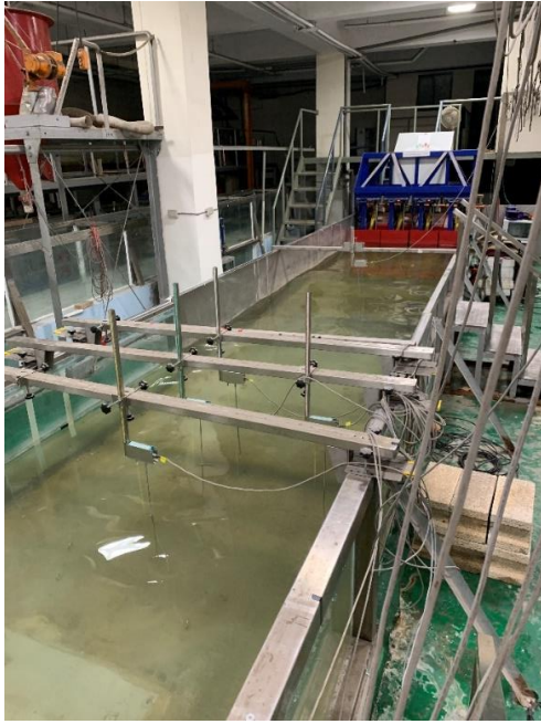
Fig. 2. Displacement piston wavemaker and wave tank
