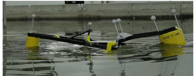
Fig. 12: Photo of the float at t = 0.4 s, at the hinge rotation trough immediately after the biggest response crest. Measured during the Design Wave test.
