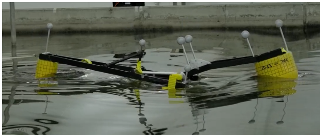
Fig. 11: Photo of the float at t = -0.6 s, at the hinge rotation trough immediately before the biggest response crest. Measured during the Design Wave test.
