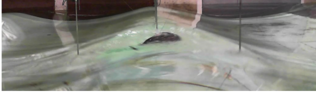
Fig. 12. Incident waves and ring wave at the sphere model in R12 for Setup 3 without reflective markers.
