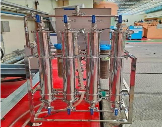
Fig. 5. Fe ions Filtering Device is now operating in Sihwa Tidal Power Plant. This device can be installed in a portable manner.
