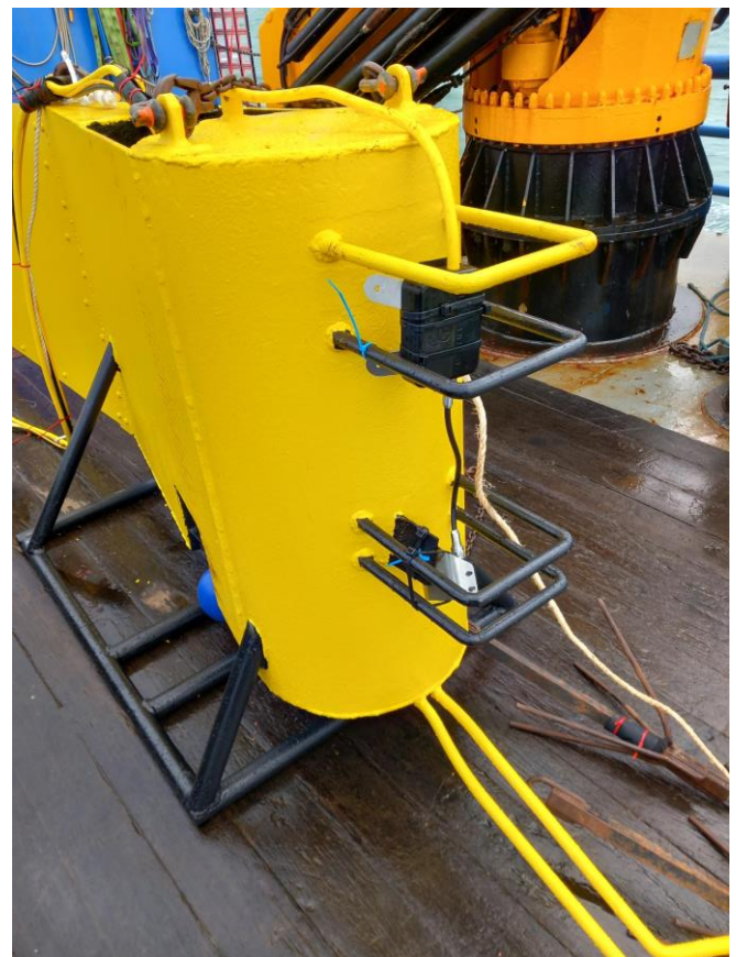
Fig. 6. EMEC's SurveyFin with dive camera, Spyball camera, and SONAR
