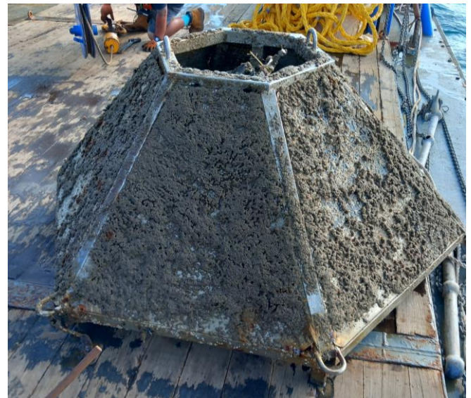
Fig. 2. ADCP frame showing marine growth from long term deployment.
