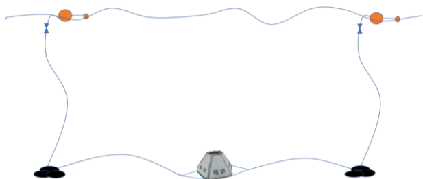
Fig. 8. U-shape configuration - ADCP, with ground lines, clump weights, and risers
