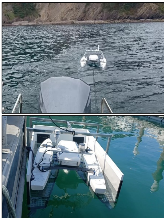
Fig. 8. ITSASDRONE towed by OLATU yacht (top), ITSASDRONE inside the docking station (bottom) (source: AZTI).
