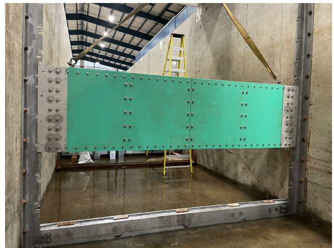
Fig. 12. Installation of the rails and panels in the Large Wave Flume.
