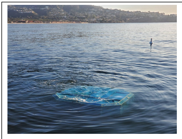
Fig. 1. CalWave XWave™ WEC as deployed in San Diego, California.
