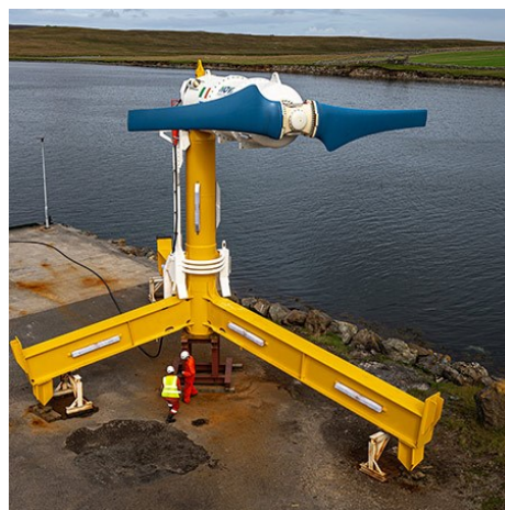
Fig. 2. Image showing size and scale of Nova's M100-D tidal turbine (Image provided by Nova Innovation Ltd.)
