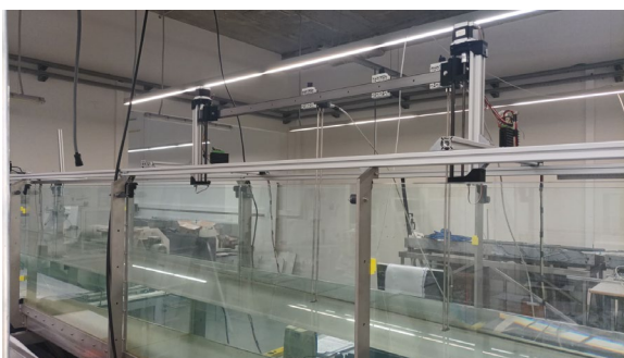
Fig 3. Overview of the automatic calibration device.
