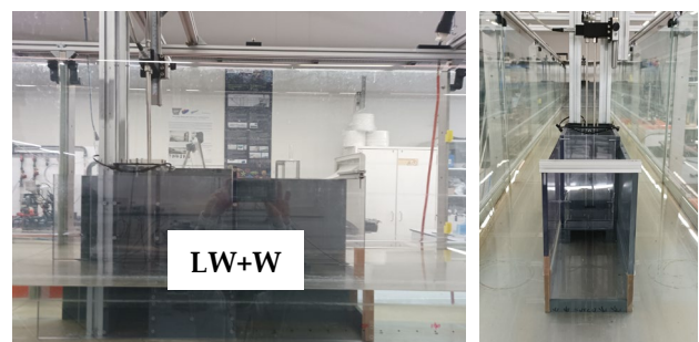
Fig. 8. Top: Tested front walls (W) with heights of 40, 80 and 120 mm. Bottom: The model inside the flume, once the Lateral Walls (LT) are joined with the W. Front view of the LW+W of 40 mm.
