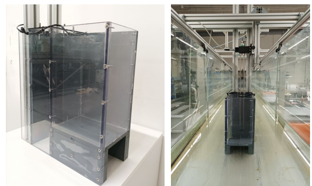
Fig. 5. a) General view of the scaled (1:36) Mutriku power plant. b) The model at the centre of the wave flume with the gauge.
