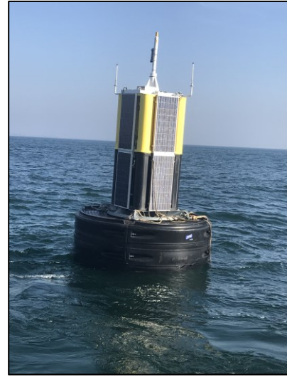
Fig. 2. The WASP deployed at the Marine Institute Galway Bay observatory, Ireland, 2019
