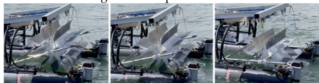
Fig.12. Automated lowering of the turbine into the water
