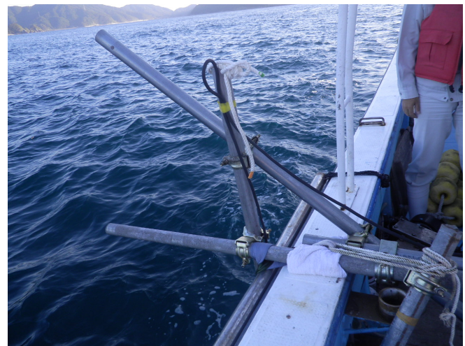
Fig. 5. ADCP-vessel attachment system.
