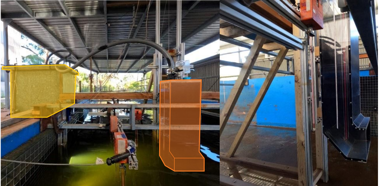
Fig. 1. Plan View of Experiment (Top); Experimental Setup showing OWC and Air Chamber (Bottom-Left); Empty Flume with OWC and rigid wooden frame (Bottom-Right)
