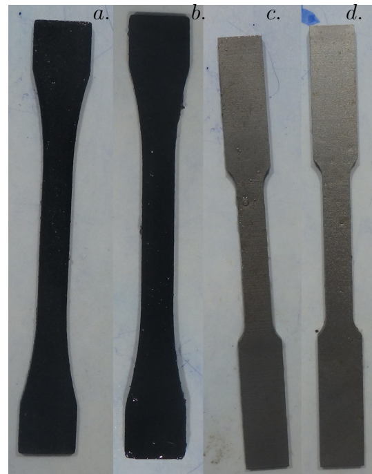
Fig. 3. Post seawater immersion: Onyx (a.), Essentium (b.), Titanium (c.) and Inconel (d.)
