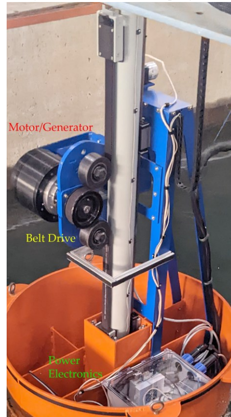
Fig. 2. Deployed LUPA power take off system. Motor/Generator and belt drive rotary to linear conversion including idler pulleys and drive sprocket.
