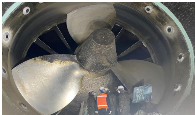
Fig. 5. Attachment of barnacles to runner blades.
