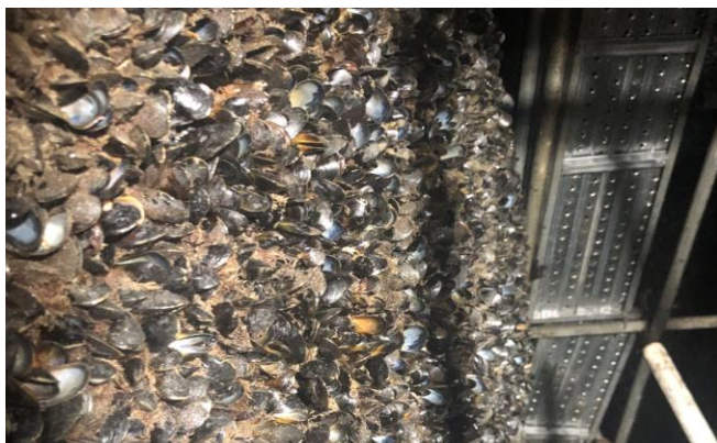
Fig. 3. Attachment of mussels to bulb case.
