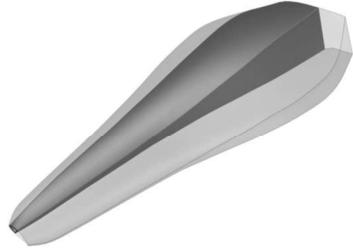
Fig. 3. Geometric definition of structural spar within the MHKF1 blade.
