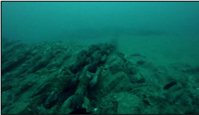
Fig. 14. Section of the shallower catenary on a rocky outcrop, at BiMEP.
