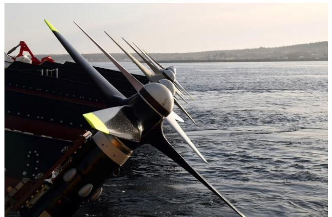
Fig. 3: SDM in raised position: turbines in parked position enabling easy access for inspection and maintenance.
