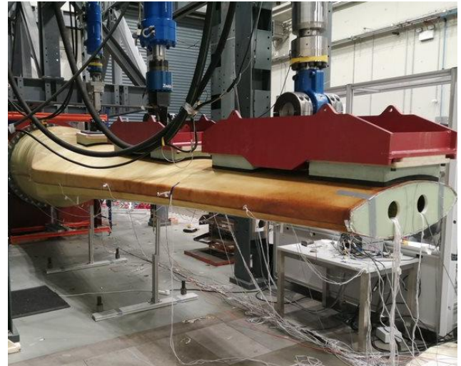
Fig. 2. Structural testing of tidal turbine blade [12]
