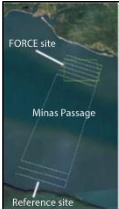
Fig. 3. Transects over the FORCE test site and a reference site used in the BACI design of FORCE's fish monitoring program.
