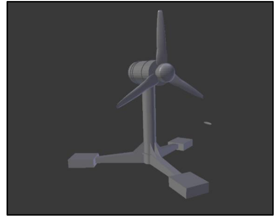
Fig. 7. Screenshot of 3D shapefile of the horizontal axis turbine design, the ellipsoid object of the seal can be seen for scale purposes.
