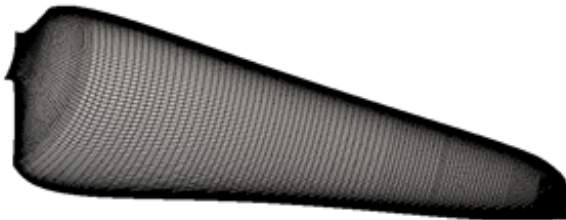
(b) Blade surface mesh
