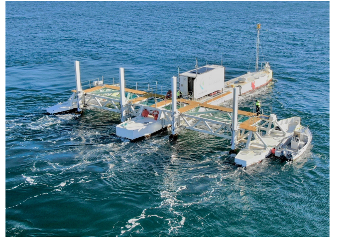
Fig. 3. PLAT-I deployed in Grand Passage, Nova Scotia. The four turbines' support structures are visible along the platform cross-deck. In this picture, turbine blades are not installed. Visible in this picture is the surface expression of the platform wake. Photo by Greg Trowse.
