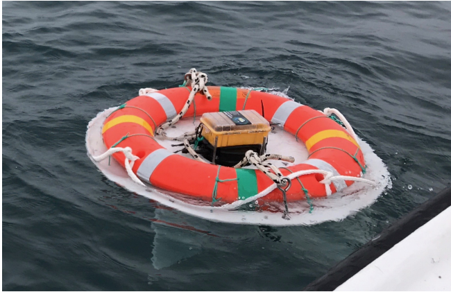
Fig. 4. Drifter buoy with GPS case and down-looking Nortek Signature 500 deployed in Grand Passage.
