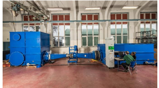
Fig. 3 Scale model, with from left to right : water tank 1, diffuser with built-in Louvre valve, pump/turbine, diffuser, frequency controller and water tank 2.
