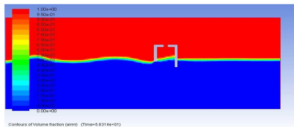
Fig. 12 shows snapshots of the water surface profile and different phases in the wave tank. In this figure, to create a free surface in the CFD program, the domain must somehow be divided into two phases of a fluid. Fluent can model the effects of open-channel flow using a Volume of Fraction (VOF) formulation, the water free surface configuration is defined as the VOF function, F = 0.5 . The wave transformations around the OWC and the wave attenuation can be carefully investigated using fig. 12 and fig. 13 shows velocity vectors and its magnitude around the OWC.
