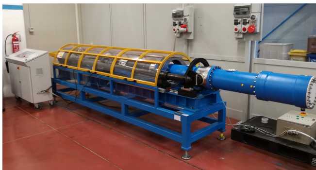
Fig. 4. Factory Acceptance Testing of the 100 kW p EMG
