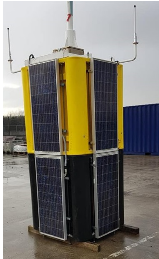
Fig. 6. Solar panels installed on the daymarks following removal of the wind turbine.
