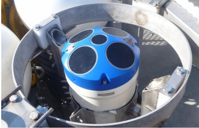
(a) BRENNIG seabed platform with one Sentinel V
