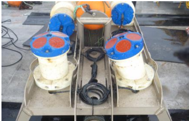
(b) MOSAIC seabed platform with two coupled ADCPs
