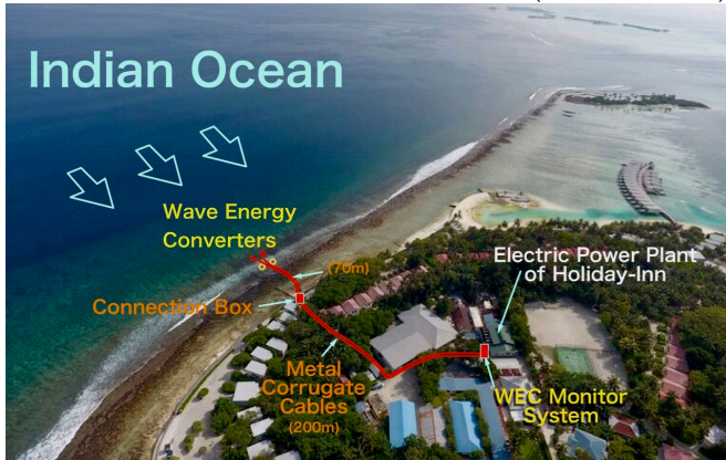
Fig.1. WEC experiment site on Kandooma Island in the Maldives. Two sets of the generators and supports were set in breaking zone. Two sets of 270m length (3.5 mm 2 , 3-lines, metal corrugate) power cables were connected to a power monitoring system, beside the power plant facility of the nearby hotel.
