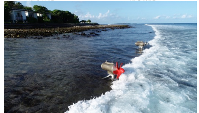
Fig.14. Full-scale 8kW generator support and socket. The turbine horizontal axis is positioned 0.6m above the sea-bed. The support socket is the same as the half-scale WECs.
