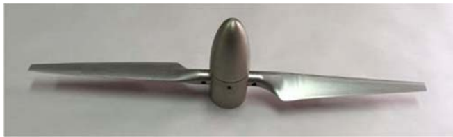
Fig. 2. Two-bladed turbine rotor and hub (800 mm diameter) with NACA 63-618 blades.
