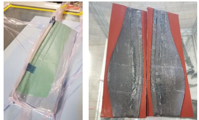
Fig. 9. (left) infusion process; (right) blade skins in mold after infusion.
