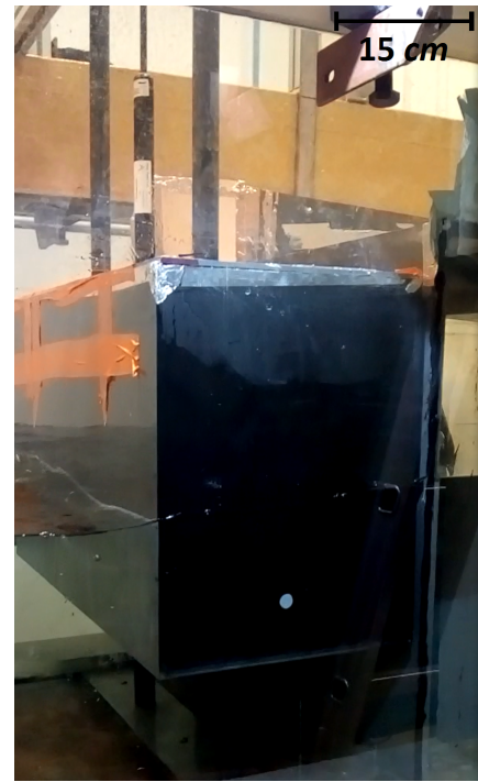
Fig. 2. Picture of one of the experimental device, with \Gamma = 0.15 m, l = 0.15 m, H_f = 0.40 m and D = 0.01 m
