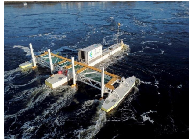
Fig. 5 PLAT-I in operation as deployed in Connel, Oban (4 m rotors)
