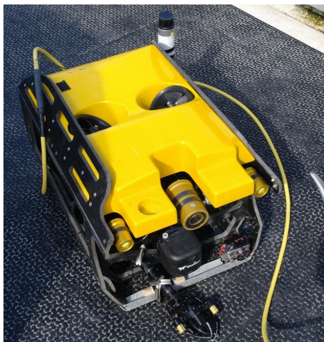
Fig. 3. ROV V4ST, attached with grabber, laser pointer, GoPro camera, high-resolution camera and tether.
