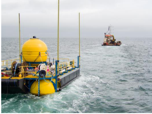
Fig. 2: Single float WaveSub on tow, showing the reaction barge in surface configuration with float docked in centre.
