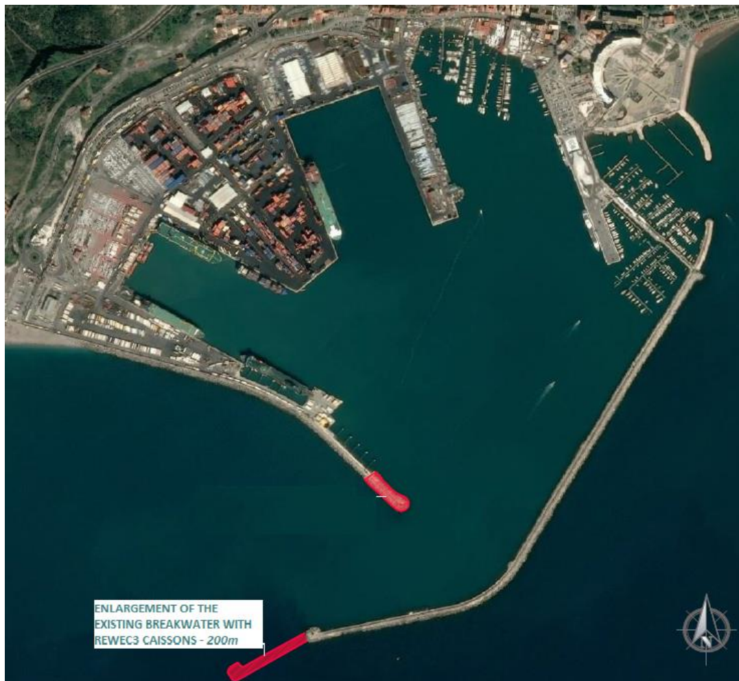
Fig. 2. Introduction of the U-OWC (REWEC3) breakwaters in the actual layout of the Port of Salerno.
