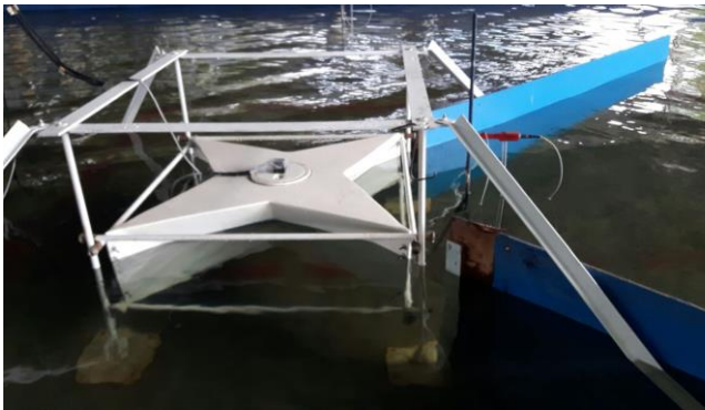
Fig. 8. 1:15 scale model test at INPH 3D basin
