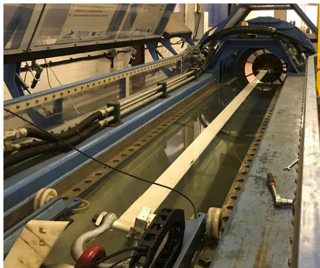
Fig. 1. Experimental setup in the Dynamic Marine Component test rig. Top figure: Engineering Drawing and conventions. Bottom figure:
