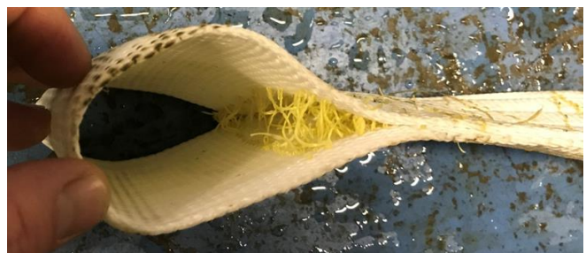
Fig. 9. Sample 1-TTS. Belt loop failure. Complete failure at headstock end (upper picture) and partial failure at tailstock end (lower picture).
