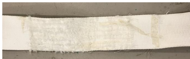
Fig. 10. Sample 3-SKB. Complete belt loop failure at MBS = 144.9 kN.
