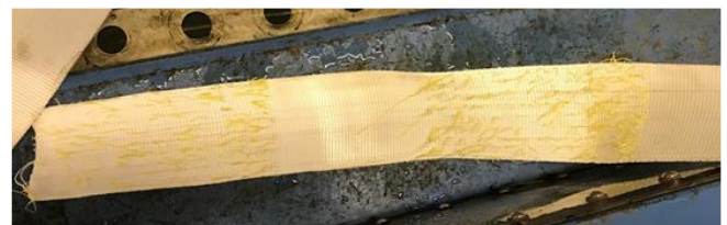
Fig. 6. Time series of tensile load test, sample 1-TTS failure at 78.0 kN. The small load slips indicate the onset of loop failure.
