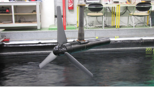
Fig. 1. Tidal turbine used for the experiment presented in Mycek et al. (2014) [4].
