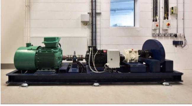
Fig. 4. The rotatory emulator connected to the microgrid.
