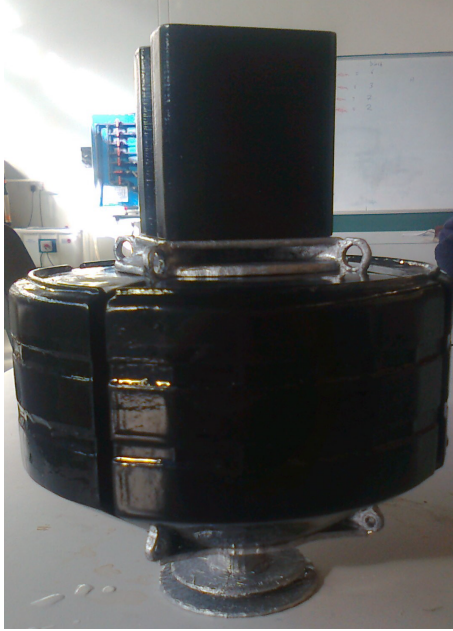
Fig. 6. 1:20 scale 3-D printed model of the WASP.
