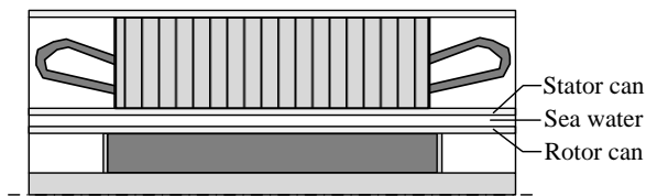
Fig. 2. Stator and rotor-can in a Flooded PM generator.
