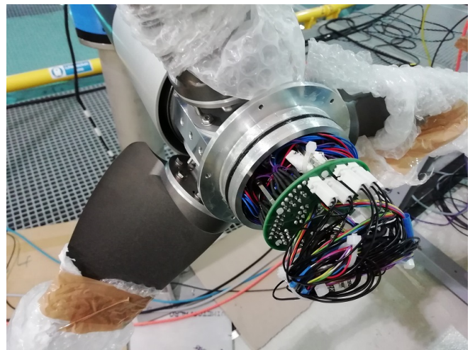
Fig. 4. Photo of nose section with nose cone and cover removed to reveal PCB for connecting strain gauges with amplifiers and connector to University of Edinburgh's nacelle.
