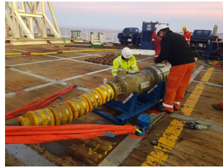
Fig. 4. D10 second dry mate connector on its guiding berth.
