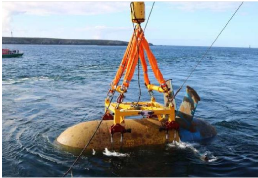
Fig. 12. D10 turbine lifting using the LARS in July 2016.
