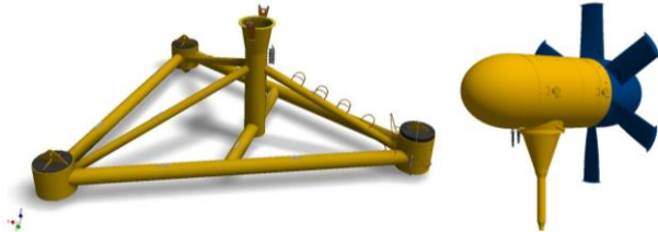
Fig. 2. Interface between the Gravity Based Foundation and the turbine.
