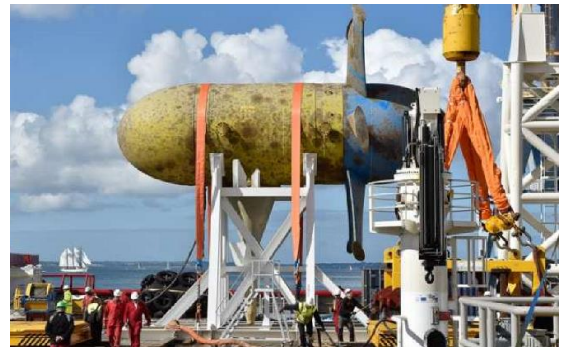
Fig. 11. D10 turbine on its offshore berth on the vessel's deck after retrieval.
