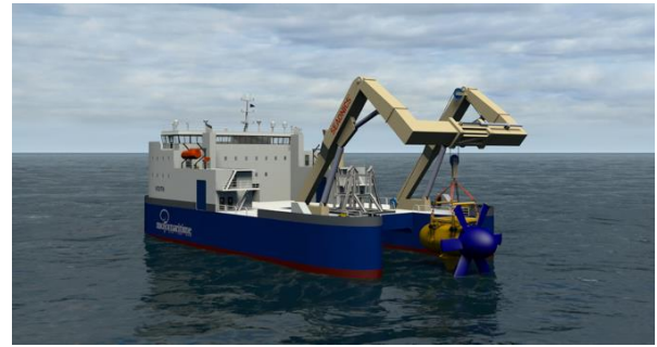
Fig. 16. Drawing of the HF4 vessel lifting D10 turbine.
