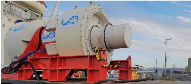
Fig. 1. Picture of the TiPA power take-off (courtesy of Nova Innovation).
