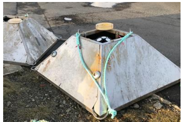
Fig 4. Stainless steel ADCP seabed frames with bullseye.
