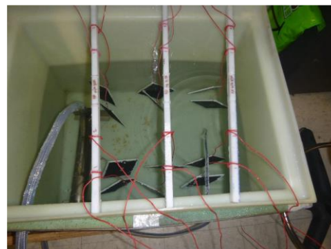
Fig. 5. Test setup for metal-carbon fiber composite interconnects at Florida Atlantic University.
