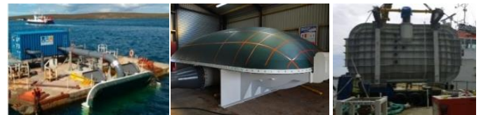
Fig. 4. AWS-III Absorber Saddle and Installation at Test Site in Scotland [32].
