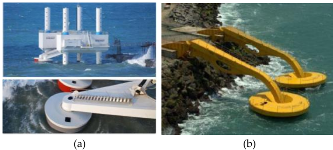
Fig. 3. Point absorbers prototypes: (a) Wave Star, with 2 floaters of 5 m diameter, rated 25 kW each, being tested at Hanstholm, Denmark, 2009 [31], (b) hyperbaric device installed at a breakwater in São Gonçalo do Amarante, Brazil, 2012. [15]
